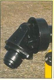
Each 3-Pt ditcher contains 2 shear bolts in the PTO should an immovable object be struck. The 3-Pt 26 also has a shear bolt\* in the wheel to protect it against damage when larger objects are hit.
