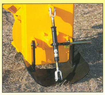
The shoe (or dragplate) on the rear of the ditcher gives the machine stability and helps prevent gouging. The shoe is also formed to the radius of the impeller to help form the ditch in loose or wet conditions. A heavy-duty ratchet jack is standard on each unit for adjustment of the shoe.
