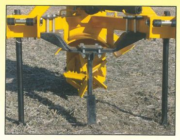
An optional ripper tooth is available on all 3 models. The tooth is designed for running in extremely hard or rocky conditions. An optional deflector shield can be used to contain the soil being distributed. The soil can be placed 4'-8' from the machine to build a diversion or small terrace.
