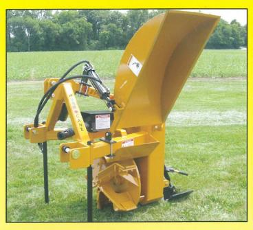
The 3-Pt 15 and 3-Pt 26 both contain a 5-paddle impeller (digging wheel). Each paddle contains hard-surfacing and is designed to be resurfaced as it wears. A deflector shield is available for the 3-Pt 15, 20, and 26 models. This shield allows the operator to control the soil if it needs to be contained for a diversion, small terrace, or simply can't be thrown.
