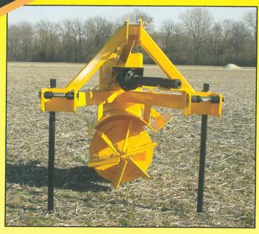
The standard 6-paddle impeller on the 3-Pt 20 can be used in any soil condition and is ideal for running in extremely trashy or wet conditions. More paddles on the impeller results in less shock on the ditcher and tractor; thus running smoother and increasing machine life.
