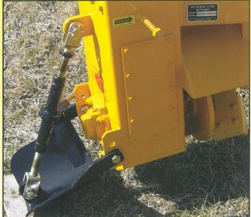
The gearbox components are easily accessible by removing the top or side cover plates. The gearbox consists of large shafts, heavy-duty sprockets and bearings, and double 80 roller chain; all enclosed and running in an oil bath. An external idler adjustment is easily accessible and should be used for chain tensioning. Proper chain tension dramatically increases the life of your equipment.
