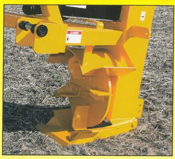
The 3-Pt 20 has an optional 18" cutting edge with shear bolts, 20" impeller and 4 replaceable hardened paddles with shear bolts. The cutting edge slices soil loose, reducing shock and vibration on the impeller and other moving parts; thus maximizing the machine's life. It also allows for multiple passes to widen or slope your ditch.
