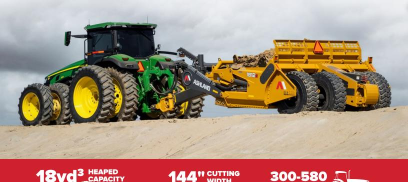
Designed using the same guiding principles as its big brothers - the Ashland high capacity construction scraper line - the 1812E packs all the same impressive performance into a smaller package, making it an ideal earthmoving solution for mid-high horsepower tractors. The 1812E has the perfect combination of width, capacity, weight transfer ratio, and ground engaging geometry to suite the needs of farmers and construction contractors doing smaller earthmoving projects.
