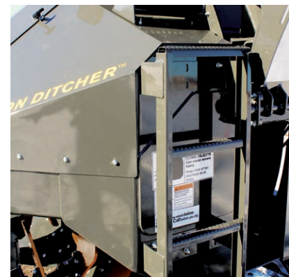
NEW ladder and steps for easy access to GPS globe and mast.
