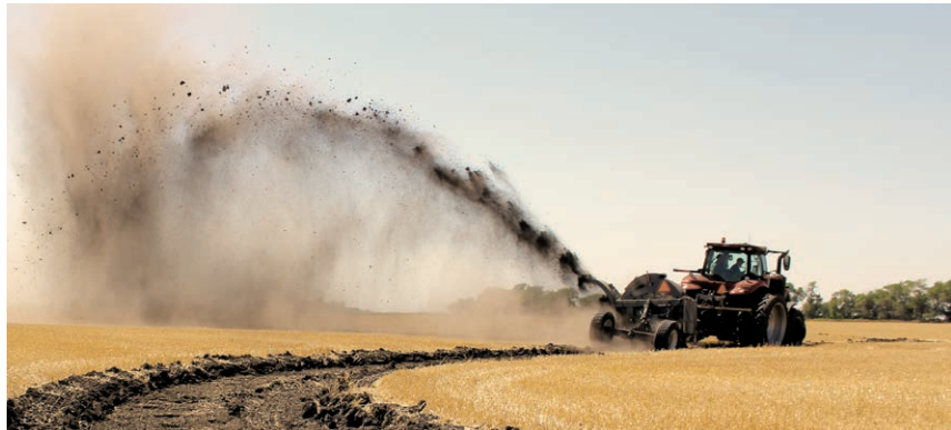
Hydraulically adjustable dirt deflector.
