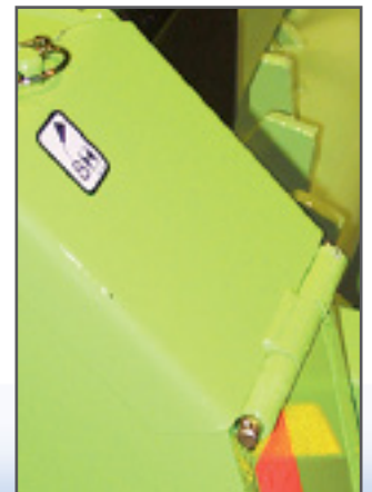
Fully enclosed final drive chain
