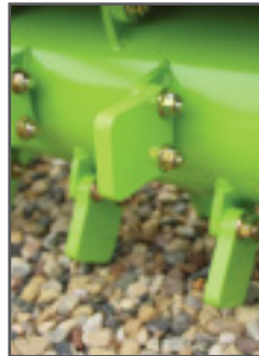
Replaceable teeth 4" & 2 1/2" 450 BHN steel
