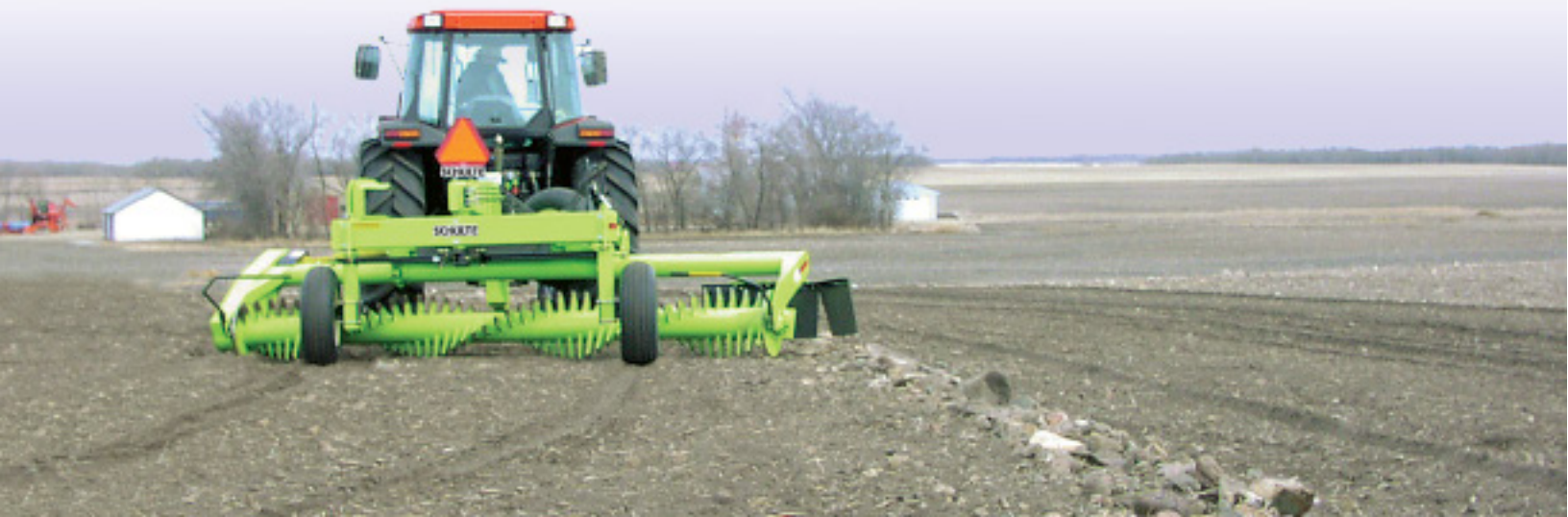
SRW-1400-H Features a hydraulic chain drive system
