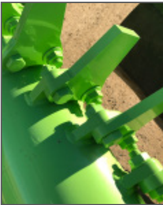
Bolt-On Replaceable Teeth
